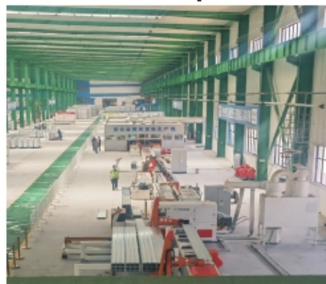
Shangjiang Group Automatic Aluminum formwork production line
